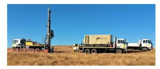
EDRS currently has a fleet of seven dedicated RC Rig outfits. The RC rigs are a combination of truck mounted (4 x 4 and 6 x 6) and track mounted rigs. Compressors and boosters are truck and trailer mounted. Drilling depths vary from 10m to 400m (depending on water intersections). All types of cyclones and splitters available.
