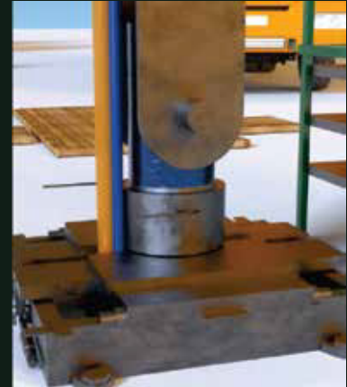
Remove the 2 Chains From the Grooves of the ZSM Coupling to Loosen the Lifting Device
